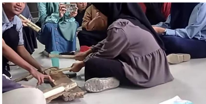
Figure 8. The process of beating the deluang bark to produce paper
